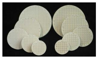
High-purity alumina-zirconia lattices are available in a range of sizes and internal lattice configurations (see sizing table) for many metals and thermal situations. Standard product sizes are 50–125mm (2–5 inches) in two grades of filtration with four flow rates per grade. Custom sizes, grades, and flow rates are also available.
