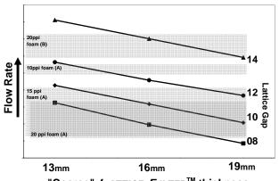
"Coarse" LATTICE FILTER™ thickness
